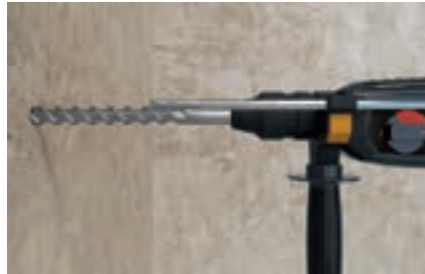
Bohren in Betonwand
